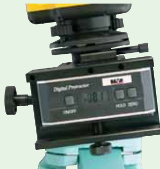
Grade mount with digital display adapter attached and digital level.
