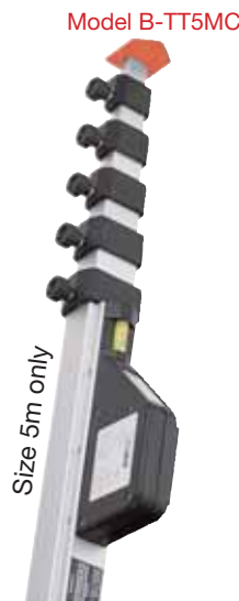
Model B-TT5MC Size 5m only The B-TT5MC (metal clamps) incorporates a positive locking screw for each section & a mm tape display that measures internal or external measurements. The red line measures under the side of the 5mm end cap, the green line measures outside of the cap. Includes carry case & horizontal bubble. Total length in closed position is 1040mm. The B-TT5MC & B-TT3M/5M/10M are all made in Europe of the highest quality aluminium & machined parts.
