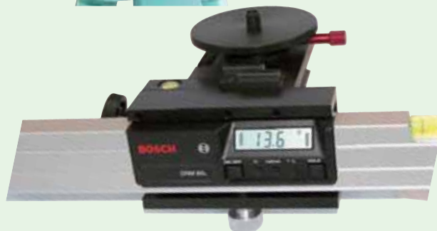
Showing grade mount and digital display adapter with 600mm building digital level.
