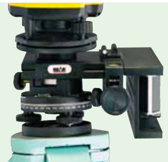
End shot showing grade mount above and digital display adapter and optional rotational base (B-360RB) Page 7.
